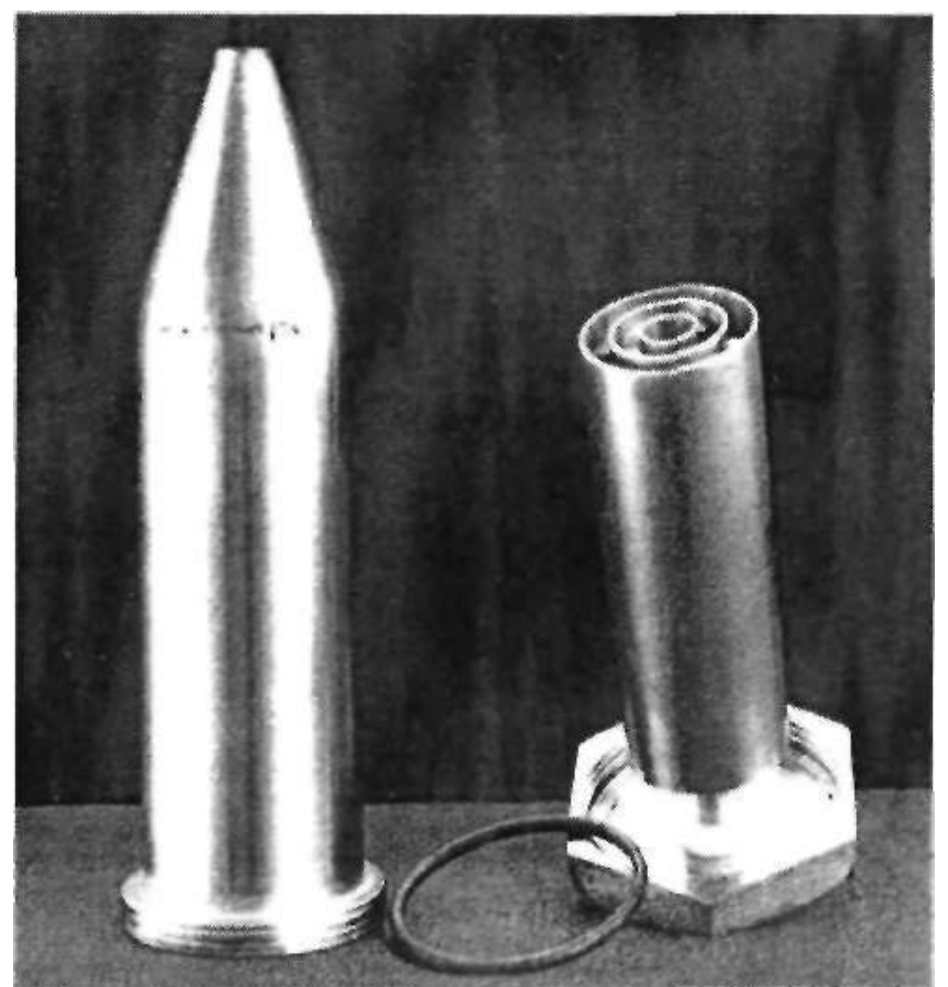
FIG 16. Cell - 4 cylinder. View of the completed cell sub-assemblies. Note that the compression fitting is missing from the top of the cone. The O-ring fits between the outer thread and
