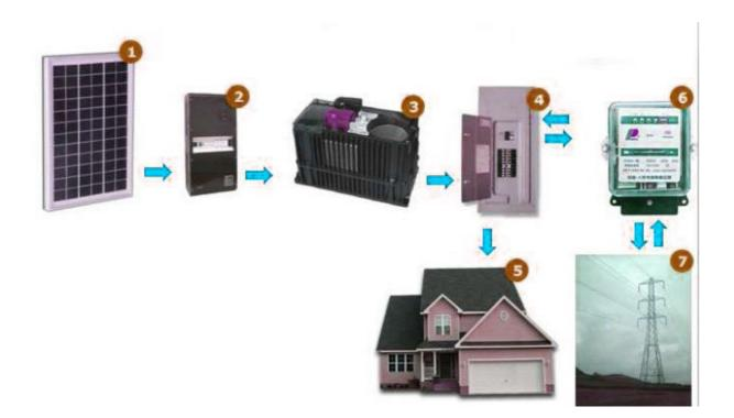
The system is also referred to as interactive solar electric system or on-grid system. It is, in fact, a conjoint system, since it entails the partial use of the local power grid. The idea is to observe what is the proportion of consumed energy to the one generated by the solar system.
