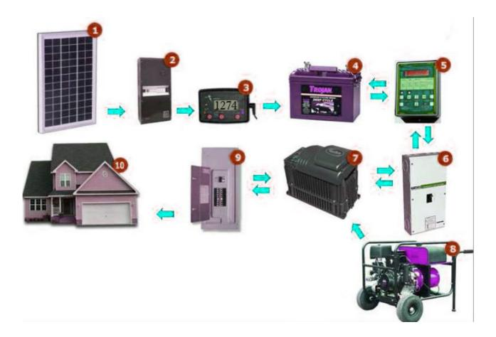
For this system, the generator is meant to undertake the function of the sun, that is, source of energy, whenever it's not available, more precisely on cloudy weather.
