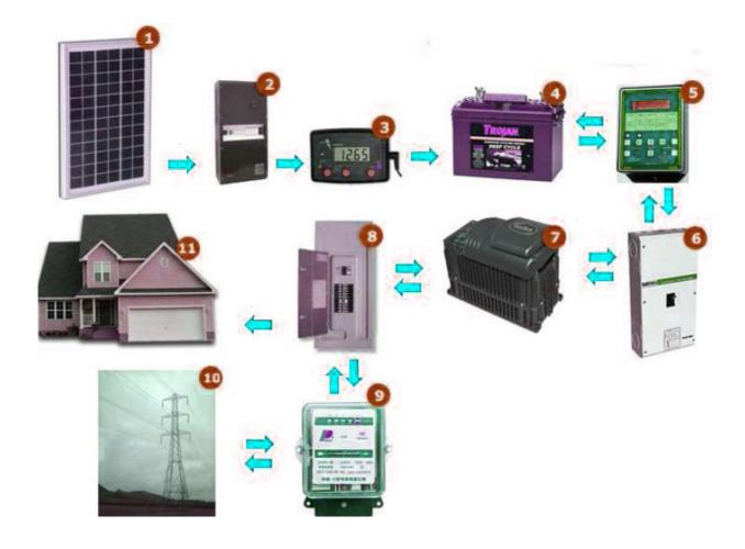
The difference between this system and the previous is that the former uses a battery backup as a solution in case the energy production is interrupted for various reasons, such as improper weather or maintenance interventions.
