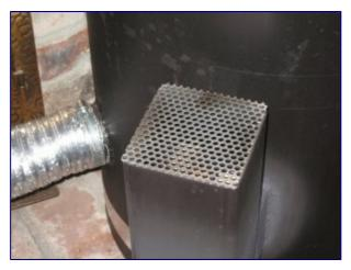
I also made a simple metal screen that can be placed over the combustion chamber to prevent sparks from popping out into the room where they could ignite something (or more likely just leave burn marks as they smolder on the carpet). I have another cover, not shown, that is a solid steel plate. It's useful to quickly extinguish the fire and to prevent air infiltration when the stove is not in use.
