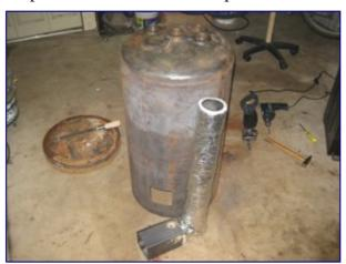
The above image shows the hot water tank cut to accept the combustion chamber and chimney.
