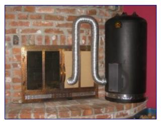
... and after a bunch more welding and a paint job that I neglected to take any pictures of ... viola! ... the finished product. The silver band around the bottom isn't a racing stripe. It covers the seam where I tack welded the bottom of the tank back on. I did not want to weld it on permanently since I may want to disassemble the stove later for inspection.
