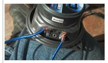
and wrapped some electrical tape around the speaker to secure the wires
