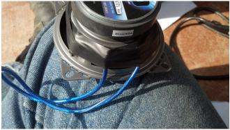
I used some sheet metal screws to mount the speakers so that they would self tap into the hard case
