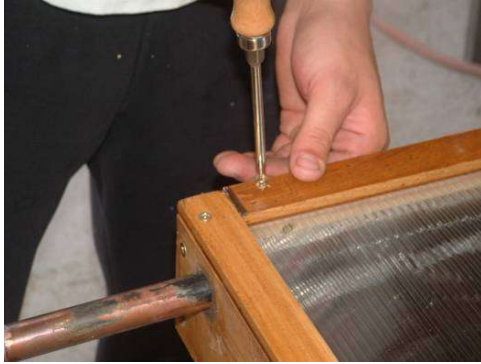
Picture 10. Fixing top beading with small screws.
