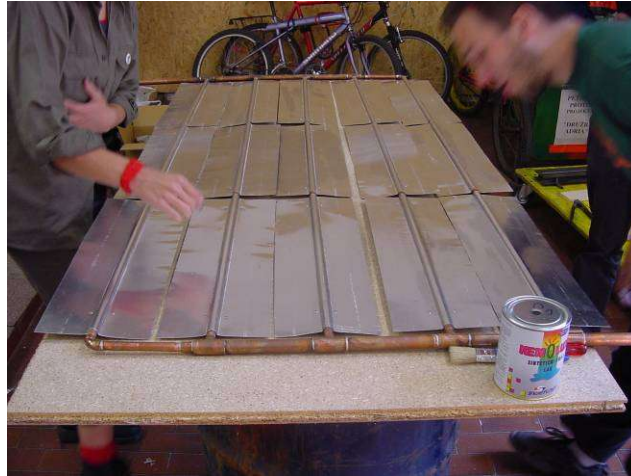
Picture 6. Completed copper matrix with attached clip fins.
