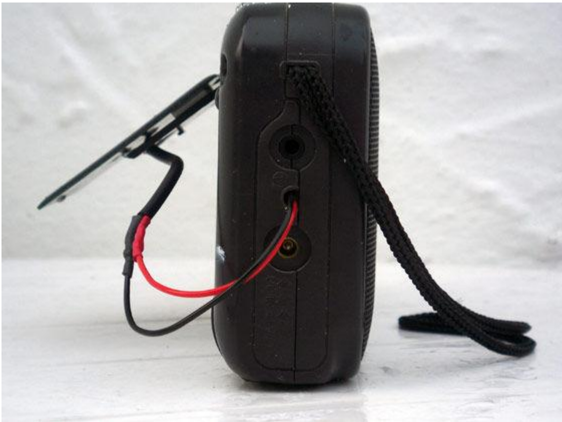
Using a piece of double sided foam adhesive tape you can position the solar panel centrally onto the radio.
