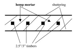
Shutterings max. 1 m. high. Once the first level is completed, fix the second level panels and apply a second layer of mortar, about 25cm. and compact. Only then may the lower panel be removed. The first level mortar has to remain enclosed for min. 30 minutes. Apply same method to the remaining levels.
