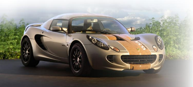
The image to the left is a Lotus 'Eco Elise' and it is constructed largely out of hemp. Everything from the door pannels to the body of the car itself is made up of the lightwieght heavy duty material. It is a stylish way to introduce this renewable resourse into the design and manufacture of automobiles. Althought Lotus can't take all the credit; Ford created the green car in the 1941 that was constructed almost entirely of hemp and ran on hemp seed.
