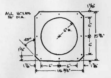
THE 16" GRID/anyway, we felt lucky to have some sheets of this so we worked out an ideal 100 per cent consistent grid pattern partially based on the reality that the actual panel size of 15 3/4"x15 3/4" would cut good out of 4'x8' plywood. i call the grid "consistent" because it can be filled in any or all of the three main directions in space without problems or compromise (or special unresolved conditions) just by adding the one-size. one-drilling-pattern universal panel.
