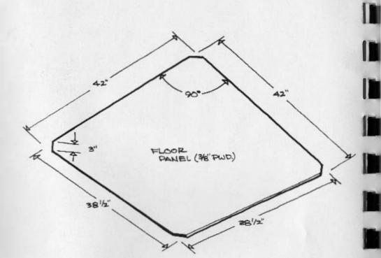
FLOOR/four separate floor panels are used. cut them as drawn, using beam compass to complete the two short sides. nip corners on a line perpendicular (90 degrees) to the diagonal. the four pieces that make up each of the four support grids are slotted together egg-crate fashion. get an accurate <u>sliding-not binding</u>-fit.
