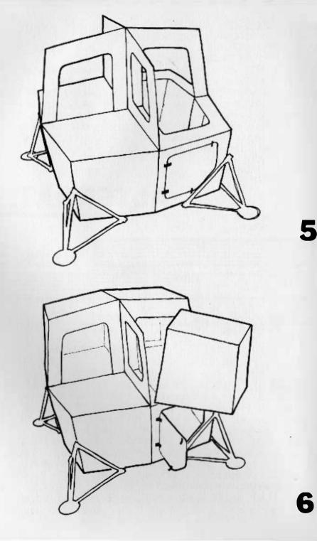
DOING THE UPPER HALF/the next operation is to get the four top inside panels bolted in place. the one between the sleeping level & the food area is a blank with no openings, but the other three have cutouts. if you have a little wind. bolt two panels that go at right angles together at their vertical joint. this will form a more stable L shape that will stand up without blowing over while you bolt it.
