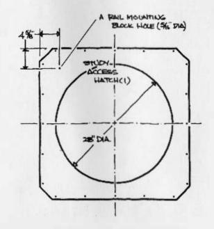
CUTTING THE PANELS/use 3/8" Douglas fir plywood (A-C faces). the eleven panels are all 35 5/8" square & can be gangcut two or three at a time with a portable electric saw & care. lay out master panel & stack securely. clamp with at least two C-clamps. guide saw against hardboard straightedge that is also clamped securely to pile. don't hurry.
