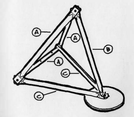
LECS TO SHELL/do a trial assembly with 3 skin panels & 3 inside panels. set assembled leg tetrahedron on this corner. use 3 mounting holes in bottom skin as guide to mark location & direction of bolt holes in bottom leg member. drill 4 of these, one for each tetrahedron.
