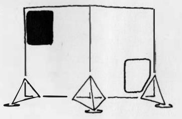
OUR MATRIX IN CHICAGO/carole & me needed some frame of reference to live in so we built four of the modules for ourselves & used them in an old North Side apartment the initial design was separated into two main assembles, the skeleton & the skin. for our use we relied more on the skeletons to preserve air circulation & openness we didn't use the skins
