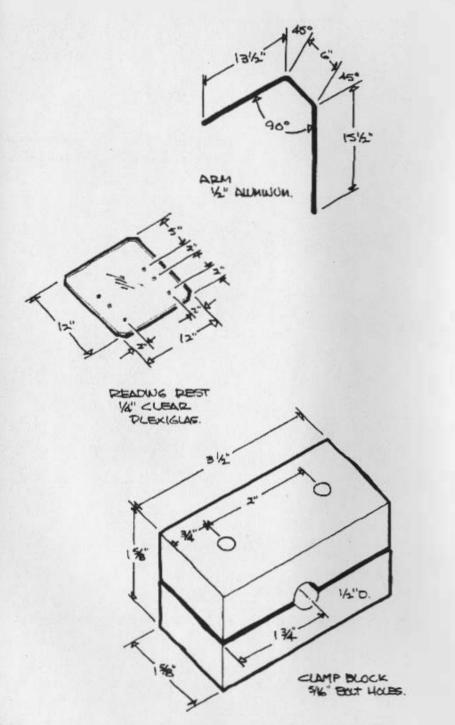
BOOKREST ARM/bend this arm from the 1/2" aluminum rod. if you want the rest to fold back parallel to the bookshelves (completely out of the way), put a 30° bend (see p. 89) in the top part. remove burrs, polish & then insert it in any of the three 1/2" holes in the right hand armrest 2x2. retain it at a good level for you by using a shaft collar above the lowest 2x2 framing member.
