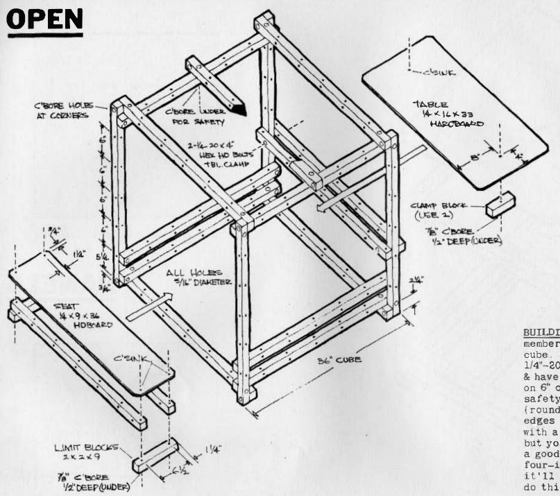
BUILDING THE ACTIVE CUBE/these members will remind you of the 24" cube. but they are assembled using 1/4"-20x2 1/2" hexagonal-head bolts & have a secondary hole pattern on 6" centers. it's a good tactile safety idea to put a 1/4" radius (rounded corners) on the long edges of the members. we do this with a high-rpm shaper (see p. 7). but you can do it with patience, a good eye & the fine side of the four-in-one rasp. don't hurry, it'll build your character. don't do this to the short edges.
