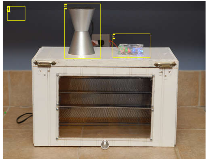
Image Notes 1. Fig.12b 2. Lava lamp base to heat the dehydrator 3. 80mm Computer fan to provide air flow
