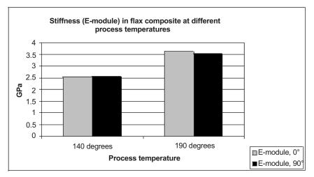
FIGURE 6. Stiffness (E-module) of flax composites at  $0^{\circ}$ , length direction of the mat and  $90^{\circ}$ , cross direction, at two process temperatures
