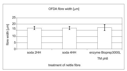
FIGURE 6. OFDA results on chemically and enzymatically separated nettle fibre collectives
