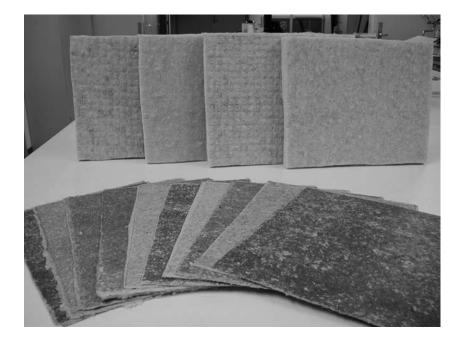
FIGURE 4. Mats and press consolidated fibre composites
