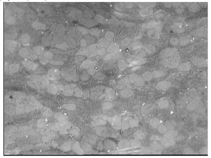
FIGURE 7B. Light microscope image of composite with semi-retted hemp and polypropylene, X31; trial no. 3
