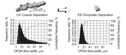
FIGURE 3. OFDA ratings on 4c bundles before and after enzyme treatment
