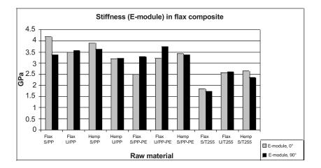
In comparison to the stiffness and strength of the fibres themselves, flax fibres obtain strength in the elementary fibre at 290 MPa in strength and 44 GPa in stiffness (Lilholt and Toftegård, 1999).
