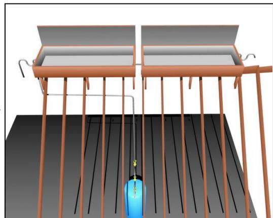
Also, if this setup doesn't coincide with the position of the sun, then it can be rotated 90 degrees and mounted so that it is perpendicular to the roof peak.
