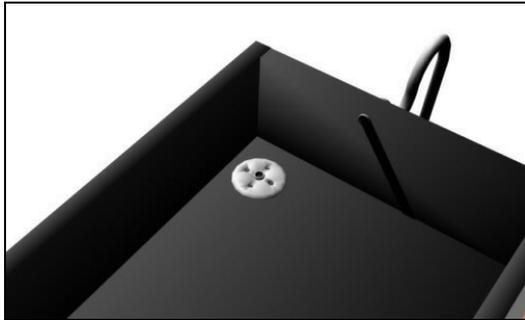
Take a piece of 4 to 6 mil black plastic and lay inside the enclosure with excess you can cut off later. In a corner of the enclosure, most convenient to running feed line to the hot water tank, drill a hole just big enough for the pipe you are using. Just cut a
