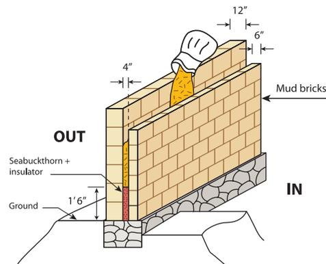
Figure 35: Plan of double wall construction
