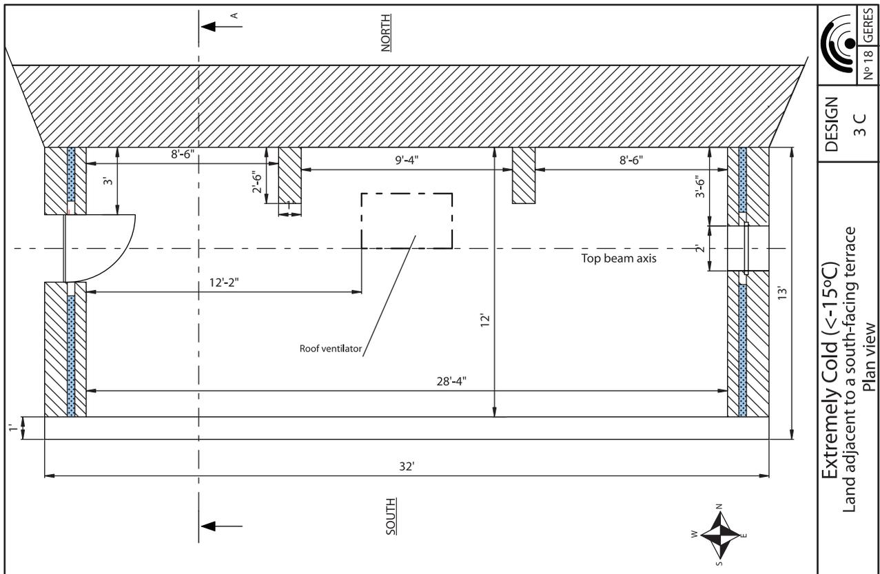
Figure 24: Design 3C - Greenhouse for extremely cold climate, site adjacent to a south-facing terrace
