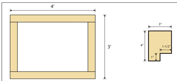
Figure 69: Construction of the frame
