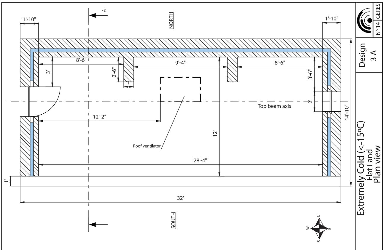
Figure 22: Design 3A - Greenhouse for extremely cold climate, flat land
