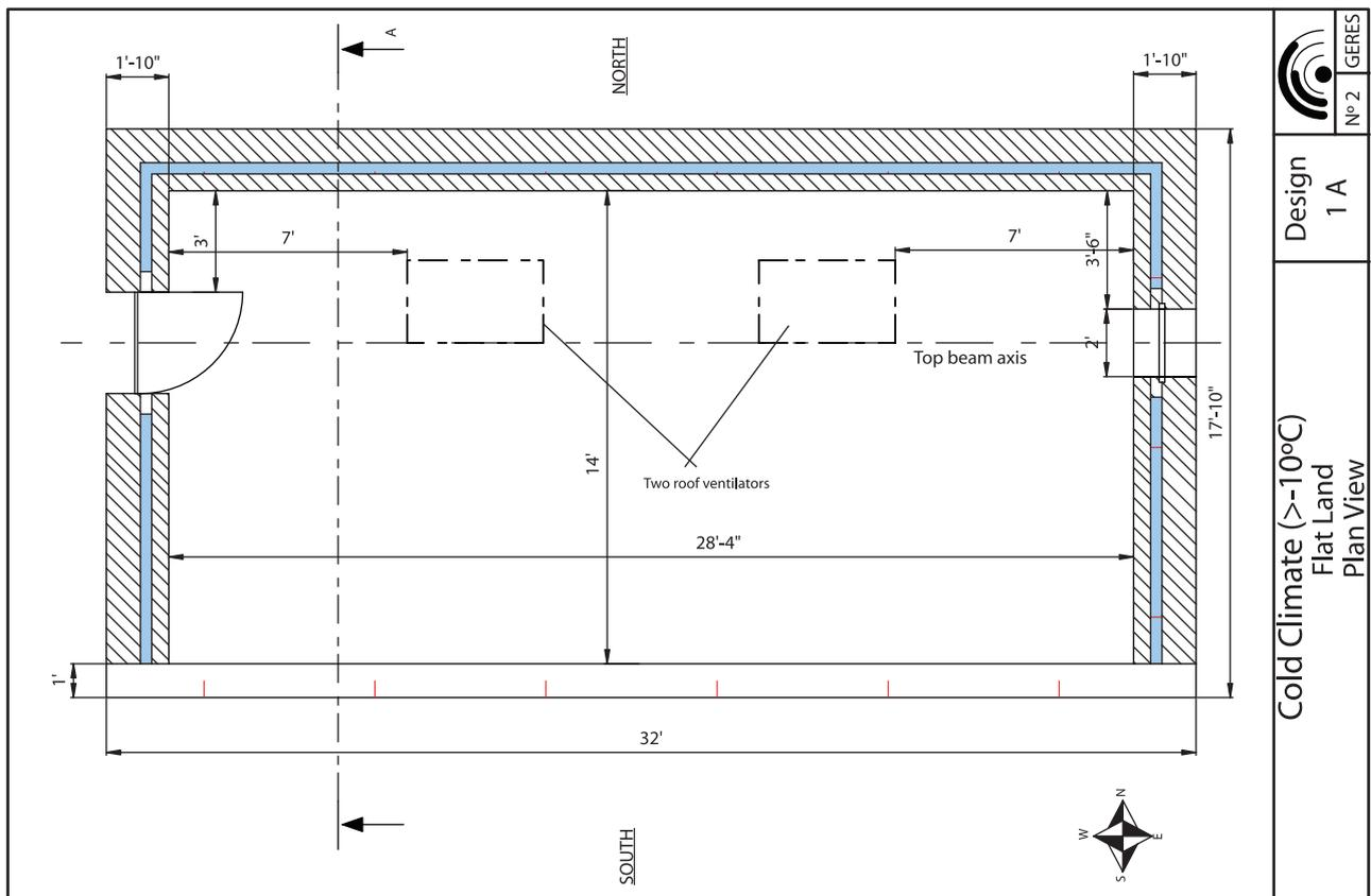
Figure 16: Design 1A - Greenhouse for cold climate, flat land
