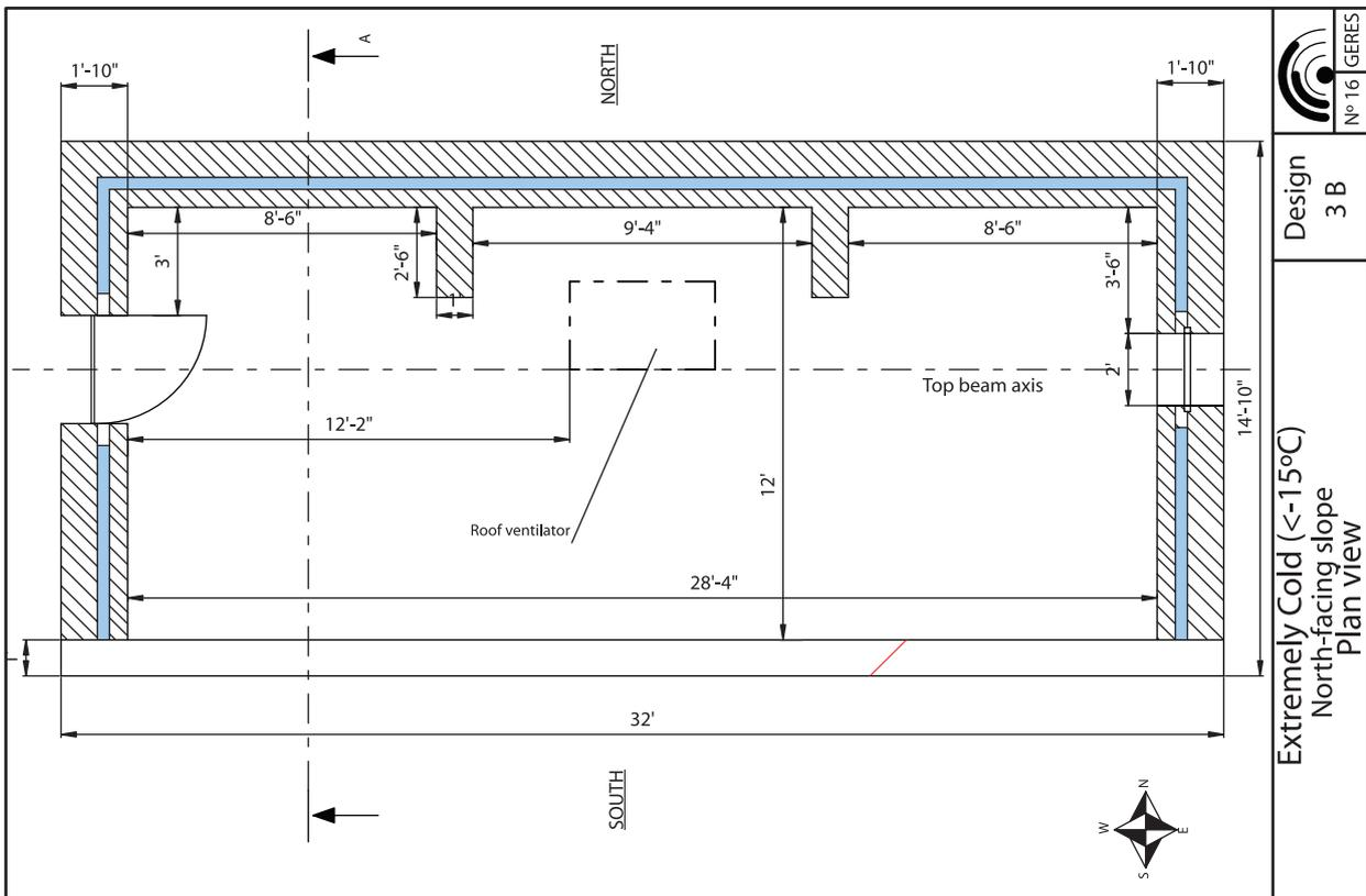
Figure 23: Design 3B - Greenhouse for extremely cold climate, south-facing slope
