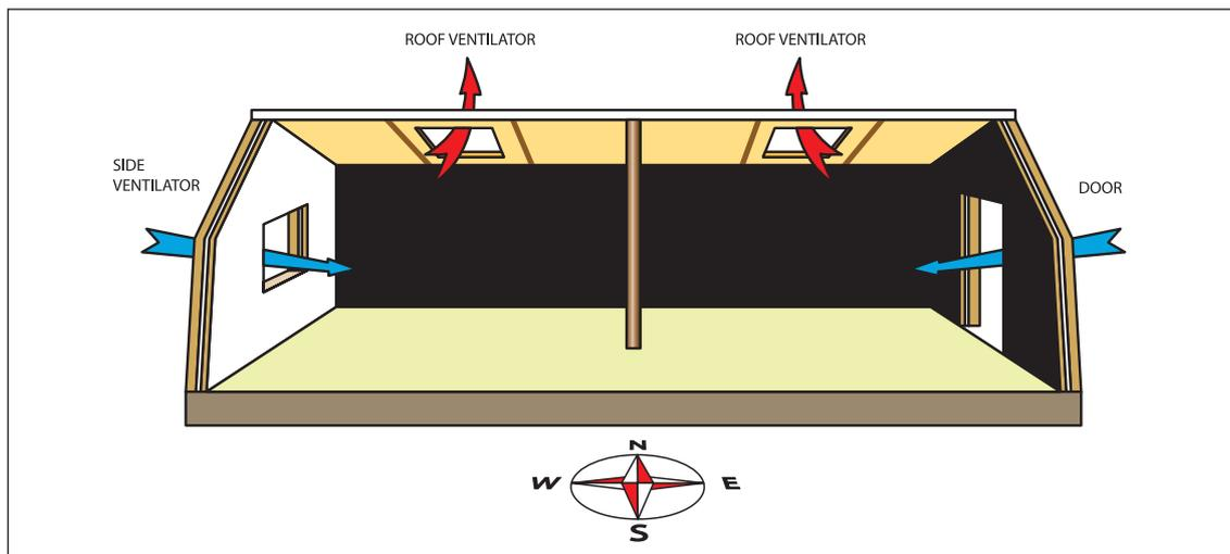
Figure 67: View of air circulation through roof ventilator
