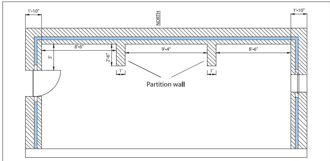
Figure 40: Plan view of greenhouse partition walls
