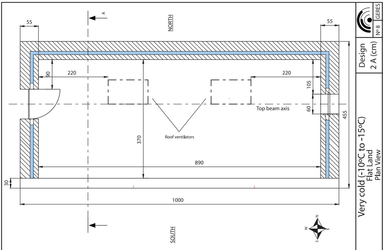
Figure 84: Design 2A (cm) - Greenhouse for very cold climate, flat land
