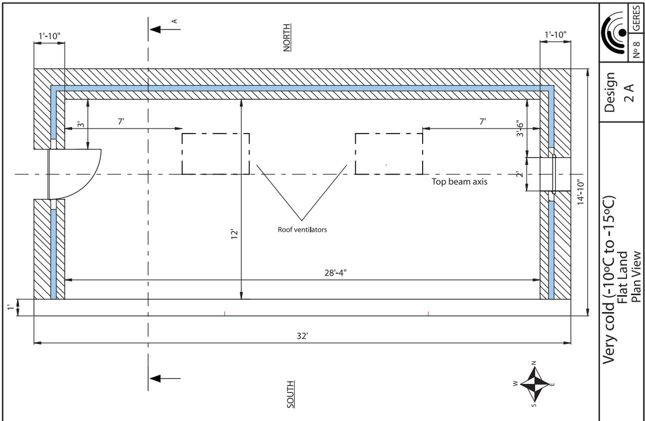
Figure 19: Design 2A - Greenhouse for very cold climate, flat land
