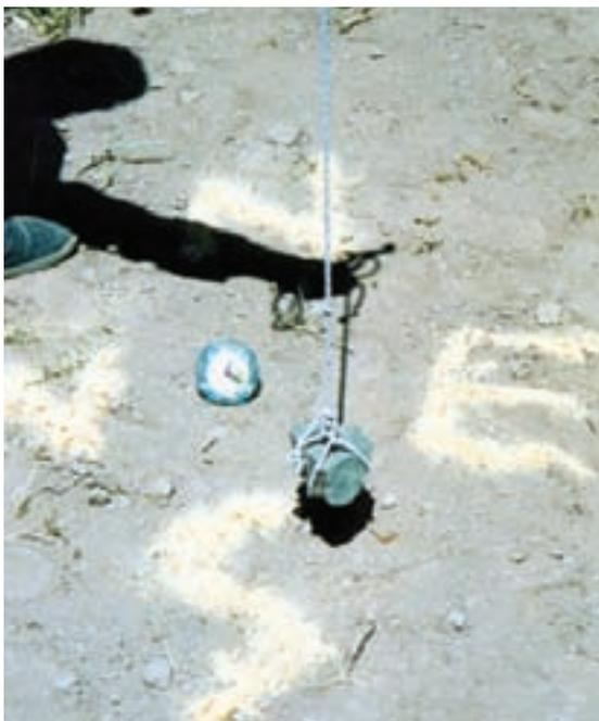
Figure 27: Finding south with a plumb line 38
