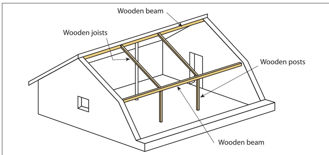
Figure 73: Wooden support structure for the polythene sheet
