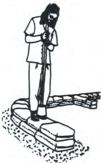
Poly bags, often used for feed, are filled with earth and tamped.
