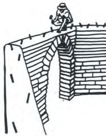
A bond beam ties walls together and provides a point of attachment for the roof.
