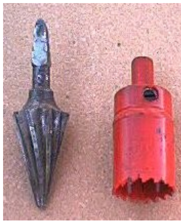
Pipe deburring tool and 1 5/16" hole saw
