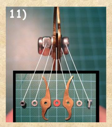
Because the ends of the two calliper claws are not exactly at the same level, you have to bent the two "claws" slightly to each other, until the points exactly meet at the same level (see pic. 12).
