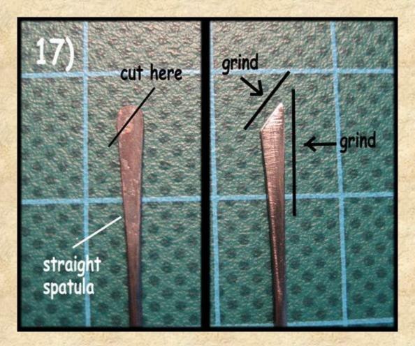
After that just make sure, to get a smooth surface on your tool tip without scratches by using the abrasive paper like I've explained before. If you are pleased with the surface, all that's left to do is to sharpen the edge of this mini knife. To do this, press the knife tip along its edge on abrasive paper with a fine grind in a 45-degree angle. Then drag it in a direction of 90-degrees to the direction of the edge, like you can see on pic. 18).
