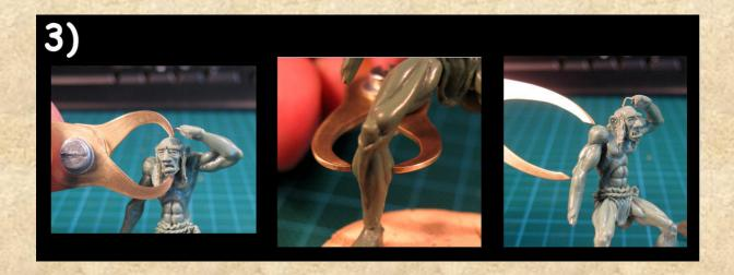
It's not difficult to build such a calliper. In short words, you just need to cut out the two "claws" of the calliper from a sheet of metal and to fix them with a bolt and nut. And that's how it goes:
