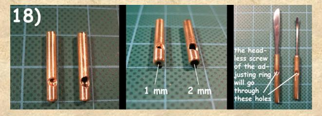
For 2mm (and 1.5-1.6mm) tool tips, I took a brass tube with an outer diameter of 3mm and an inner diameter of 2mm (material strength: 0.5mm).
