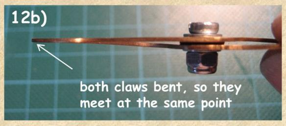
Screw the nut and bolt as tight that there is some resistance while opening and closing the callipers claws while they can still be moved smoothly.
