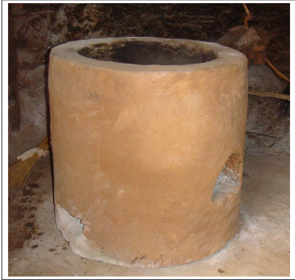
Photo 5: A typical shielded fire stove
