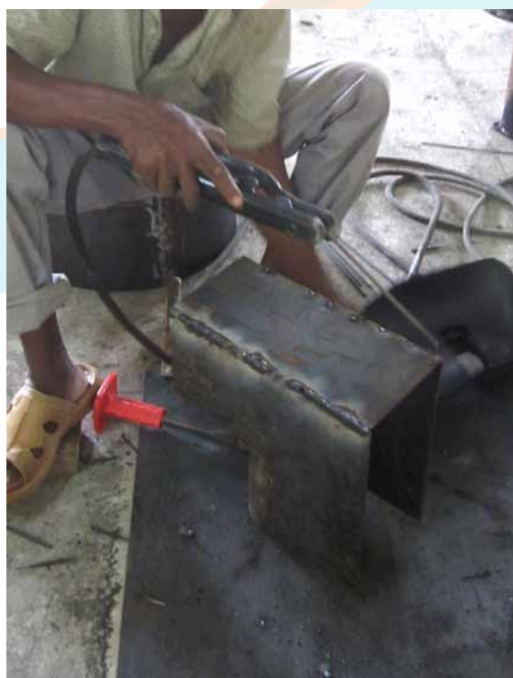
Photos showing the welding of the 'elbow' shaped combustion chamber.
