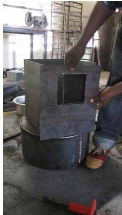
An illustration and photograph showing the outer casing assembly.
