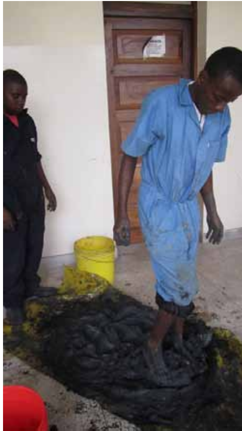
Photo showing the mixing by foot of clay, charcoal and sawdust
