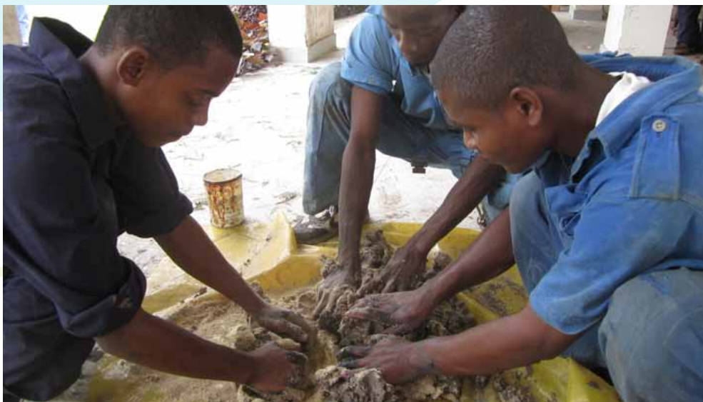
Photo showing the hand-mixing of clay and sawdust
