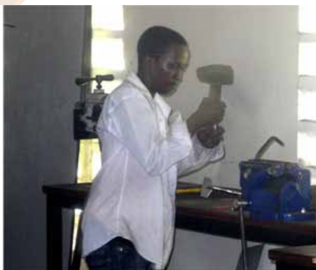
Photos showing the bending of the support brackets using a hammer and vice
