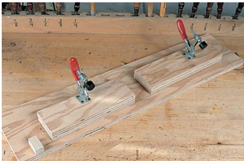
A simple jig for tapering on the bandsaw.
