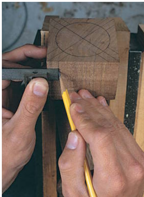
A combination square excels at transferring dimensions, especially in multiple parts.
