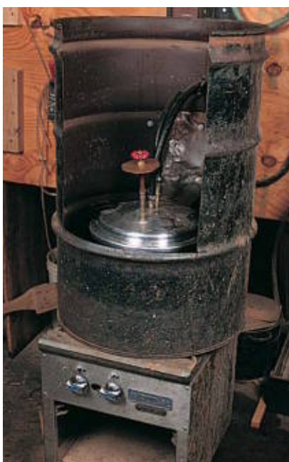
A pressure cooker mounted over a gas stove provides steam for wood bending.
