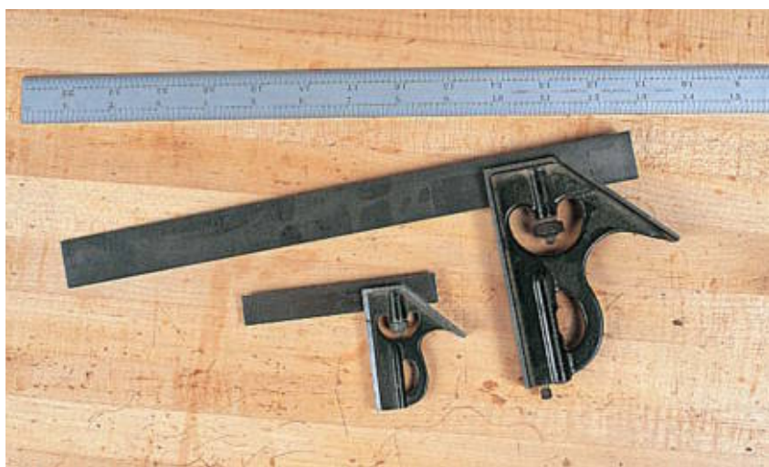
Basic layout tools include a steel rule with gradations to \frac{1}{64} in. and a reliable combination square.
