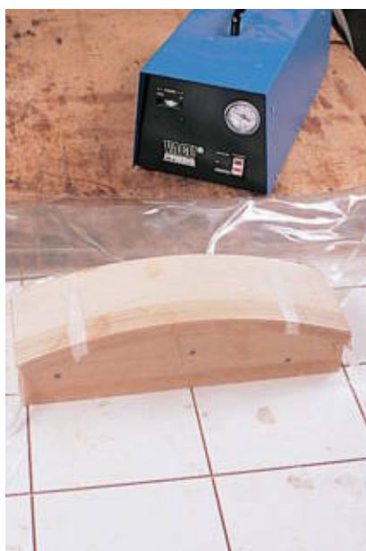
A vacuum press is normally used for veneering but is also an efficient way to make bent laminations.
