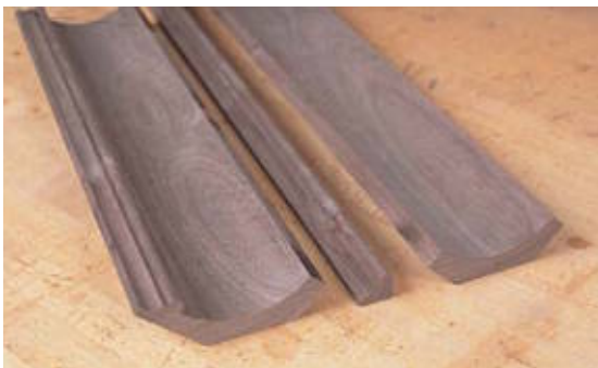
Coves are an important element in the design of crown moldings. This complex example uses two coves.
