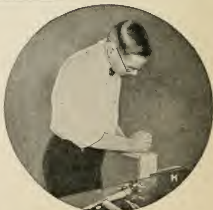
FIG. 31.—How to make a multiple dovetail joint of the type used in drawers. This is often called a "lapped" dovetail because the joint does not show from the front. It is one of the strongest and most craftsmanlike joints.
