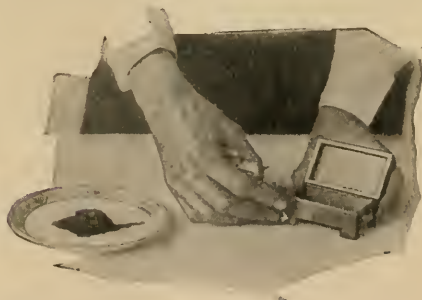
FIG. 8.—Dusting gold bronzing powder on a jewel box previously coated with japan gold size.
