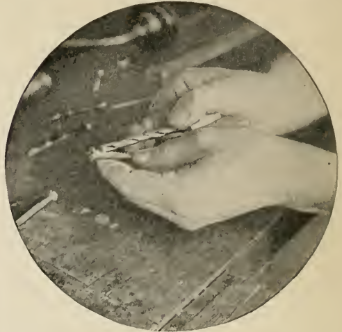
FIG. 14.—Placing the bit on the shank of the screw to obtain the correct size before boring.
