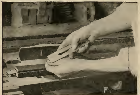
FIG. 1.—Steps in sharpening chisels, plane irons, and other chisel-edged cutters. How the keenness of the edge may be tested on the thumb nail.
