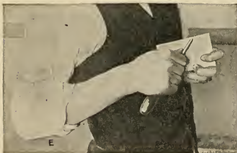
FIG. 8.—Steps in sharpening a cabinet scraper, first by draw filing, second by rubbing it on an oilstone, and third by burnishing it. How a scraper is held in actual use.
