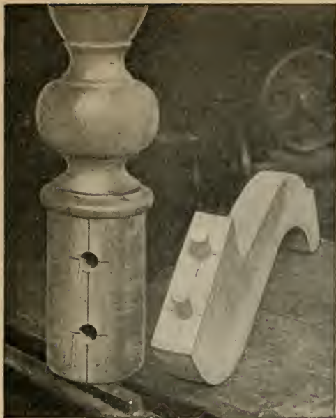
FIG. 33.—One of the legs with dowels inserted, all ready to be glued to the turned column.
