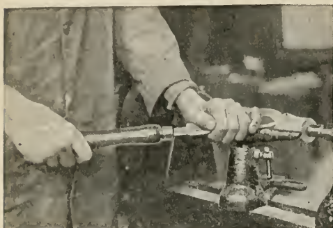
FIG. 17.—Start the cut near the dead center and move the tool toward it. Hold the tool as illustrated and stand in the position shown.
