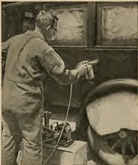
FIG. 4.—The sprayer should be held at about 8 in. from the work and kept in motion at all times.
