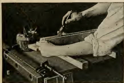
FIG. 23.—How to glue boards together: arranging them, planing, testing for trueness, applying the glue, and clamping.
