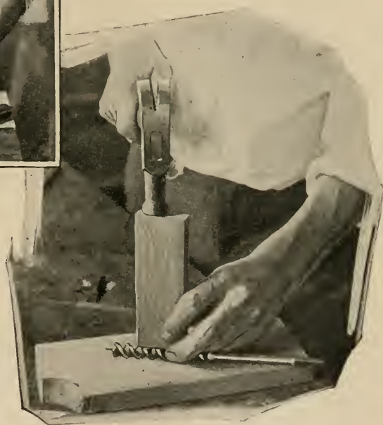
FIG. 6.—Doctoring the screw point with an oilstone (usually called a "slip") that has a thin edge.
