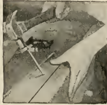
FIG. 14.—Placing the bit on the shank of the screw to obtain the correct size before boring.
