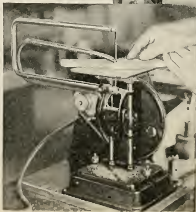
FIG. 16 (at left).—Cutting the inside of the handle on the jig saw is as simple as guiding a sewing machine.
