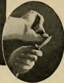
FIG. 10 (below).—The thumb-nail method of testing sharpness.
