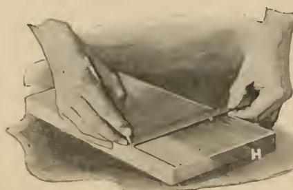
FIG. 24.—Steps in planing a board accurately. Testing the surface and ends for trueness, gaging for thickness, sawing off to length, and marking for width.
