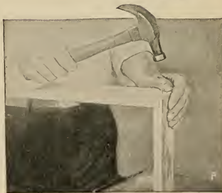
FIG. 27.—Rabbeted joints. How to measure and mark the width and depth of the rabbet, saw out the surplus wood, and nail the boards together.
