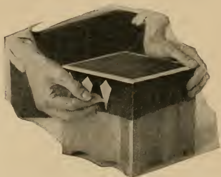
FIG. 7.—Gummed tape is used to make masks for shielding certain parts of the design before painting.
