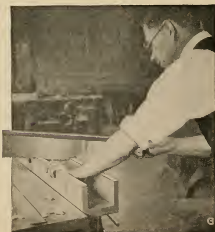
FIG. 19.—Steps in making a miter box of wood. The work must be done with extreme care, and the cuts should be made with the saw which is to be used with the box.
