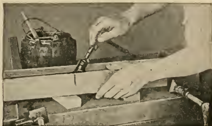
FIG. 20.—Hot glue always should be applied freely to both edges of the wood to be joined.
