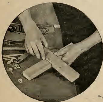
FIG. 29.—Illustrating a good method of making a cross-lap joint. Squaring and face-marking the pieces, gaging and marking the depth of the lap with a gage, making the saw cuts to the knife lines, chiseling out the waste wood, and lapping the joint together.
