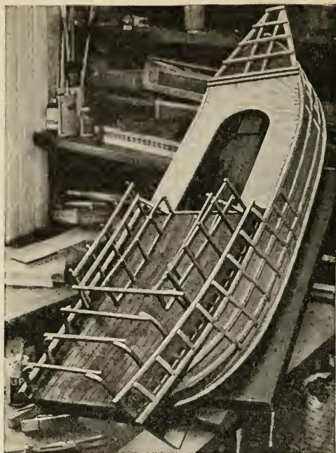
FIG. 29.—The strips for supporting the forecastle, and the framework for the stern superstructure.
