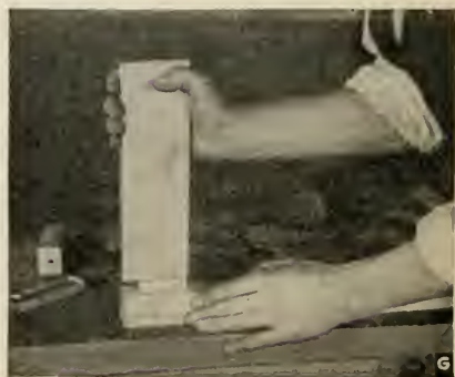
FIG. 28.—Steps in making a mortise and tenon joint. How to gage and mark the mortise and tenon in the leg and rail of a table; using the auger bit and chisel to make the mortise, and the rip saw to cut the tenon; pressing the finished joint together.
