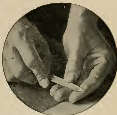
FIG. 46.—How the point of a file is ground for drilling glass.
