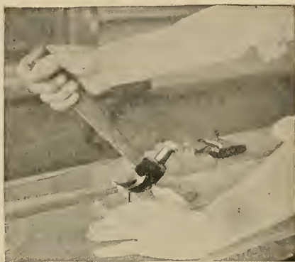
FIG. 11.—A block under the claws of the hammer is necessary in drawing long nails.
