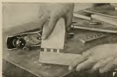
FIG. 26.—How to make doweled butt joints. Gaging and marking for the dowel holes, boring them, making the dowels, and testing the joint.
