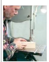
A band saw has a long, thin blade welded into a loop. An electric motor powers the blade around two large wheels.
