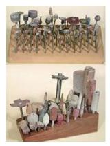
A wide variety of burs are available to fit the several different styles and sizes of Foredom hand pieces. Burs that may have been intended for other purposes can be used for woodcarving, such as single cut and double cut carbide burs (intended for metal work).
