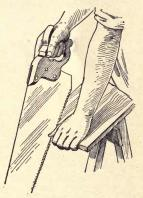
Fig. 14-Guiding the Saw with Left Thumb
