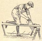
Fig. 15- Correct Angle of Saw
