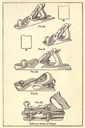
be cut off before the plane iron can touch the low places. Its iron is sharpened like that of the smooth plane—straight across.
