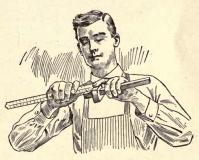
Fig. 36- Holding and Setting Marking Gauge
