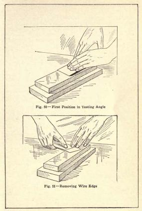
over the cutting edge will reveal a "wire edge." This must be removed before the iron is used again. To do this, hold the plane iron, face down, so that it touches the stone along its whole length, and give it a forward and downward movement on to the stone (Fig. 51). This generally bends the wire edge under and cuts it
