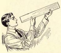
Fig. 32-Sighting for Straightness of Edge
