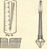
Fig. 79-Countersunk Hole and a Countersink
