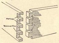
Fig 118-Dovetail Joint
