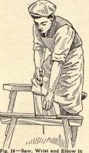
ig. 16-Saw, Wrist and Elbow in One Plane ish of a cut, lessen the length of the stroke and hold up on the saw so that little weight rests upon the
