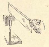
Fig. 120-Sawing the Mortises
