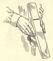
Fig. 26-Adjusting the Plane Iron
