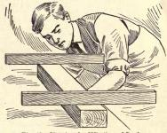
Fig. 45-Sighting for Winding of Surface
