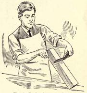
Fig. 47-Testing Across the Grain
