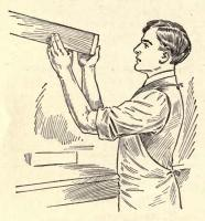
Fig. 43- Testing for Straightness
