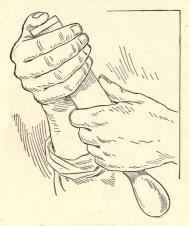
Fig. 52 - Testing for Sharpness
