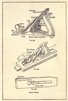
the Y-adjustment in the slot in the cap iron made for it. Next, place the cap in position and push down the cam. Should this cam work loosely and the plane iron and cap iron not be held firmly, adjust the cap screw. Ordinarily this screw when once adjusted needs no
