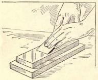
Fig. 49- Proper Pitch of Iron
